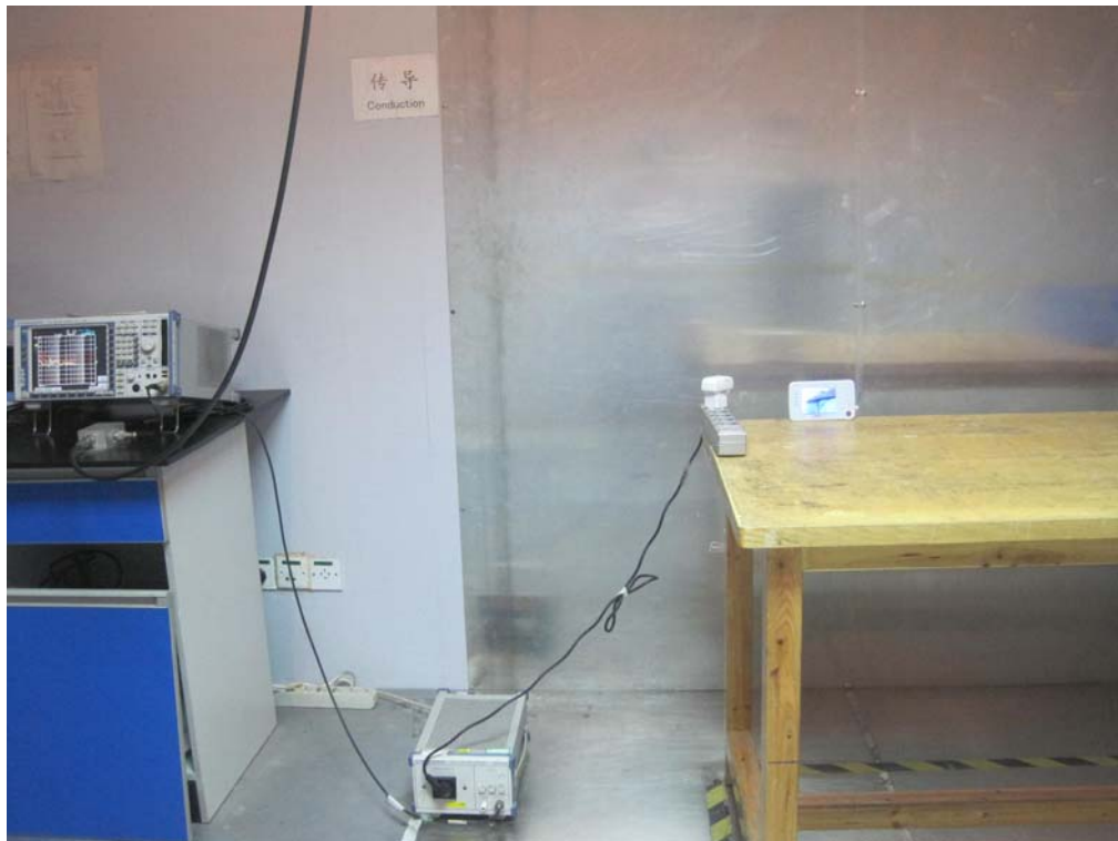
Photograph – Conducted Emission Test Setup
