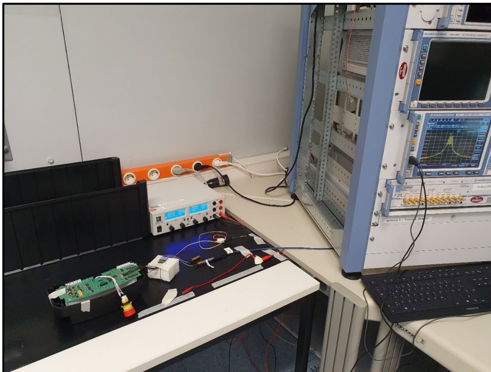
Photo 23: Conducted Test Setup - EUT Overview Port X14 (Port X11 terminated with a 50 \Omega )
