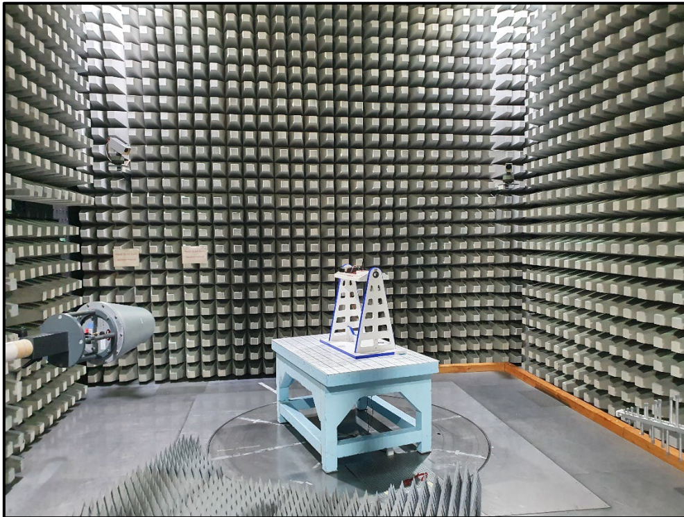
Photo 10: Radiated Test Setup-1 GHz to 18 GHz – Rod Antenna
