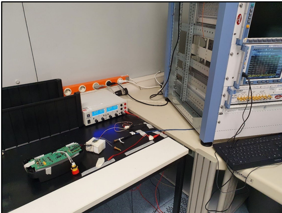
Photo 21: Conducted Test Setup - EUT Overview Port X11 (Port X14 terminated with a 50 \Omega )
