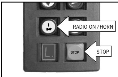
Safety equipment in the NBB-radio remote control:
