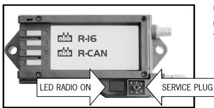
Checking the LED at the receiver R-16 and R-CAN:
