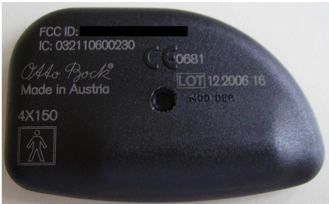
The FCC ID label is realized using a laser marker on the bottom side of the case.
