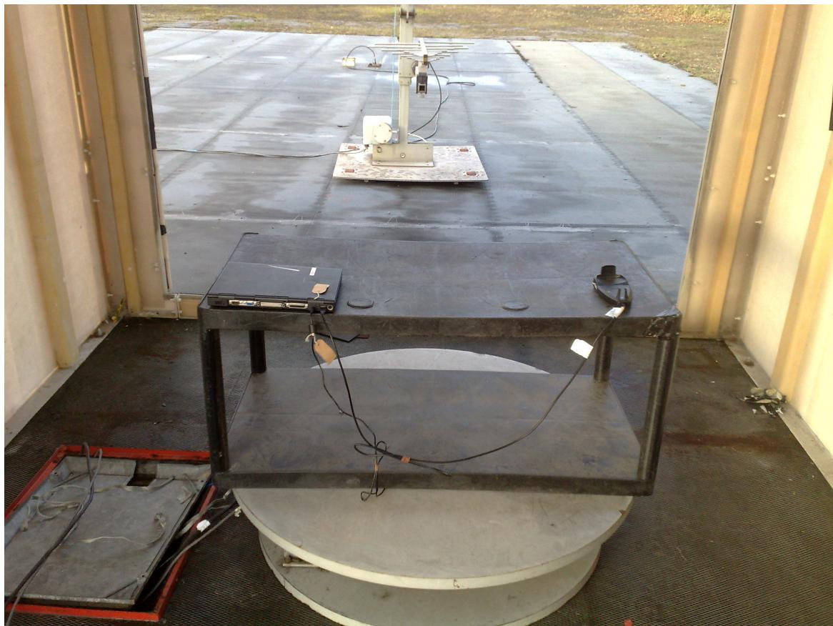
**Radiated Emissions Test Configuration 9kHz – 30MHz**
