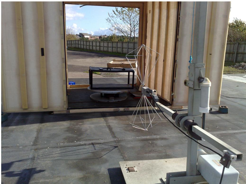
**Radiated Emissions Test Configuration 9kHz - 30MHz**
