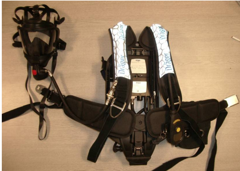
PSS7000 EMU fitted to compressed air breathing equipment
