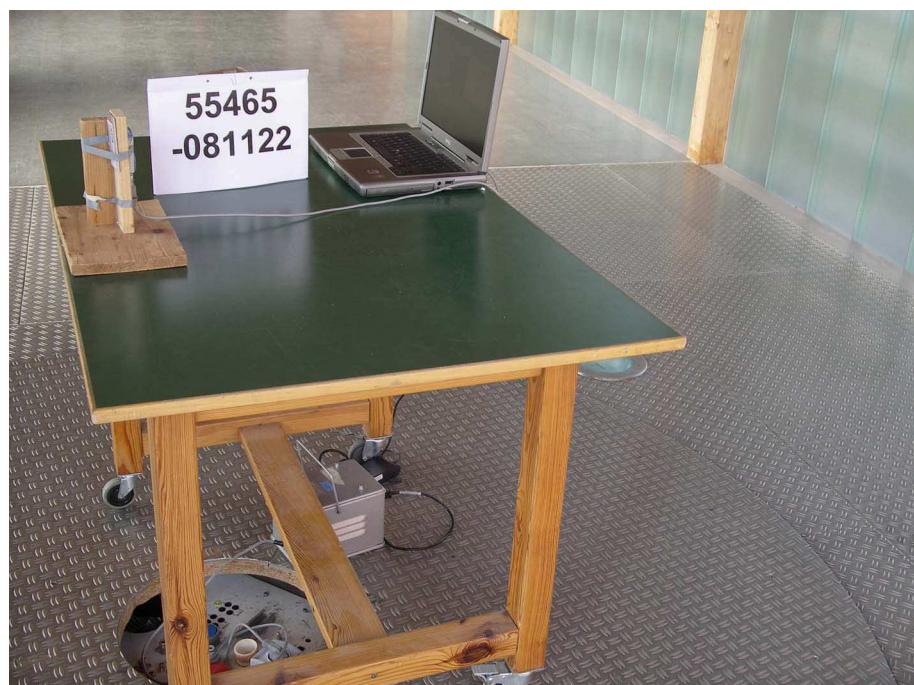
**Test setup for radiated emission measurement
