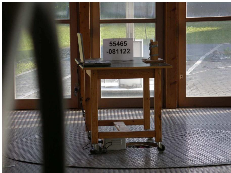
**Test setup for radiated emission measurement
