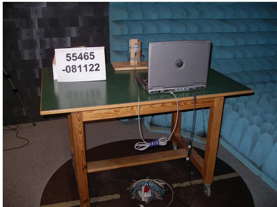
**Test setup for radiated emission measurement
