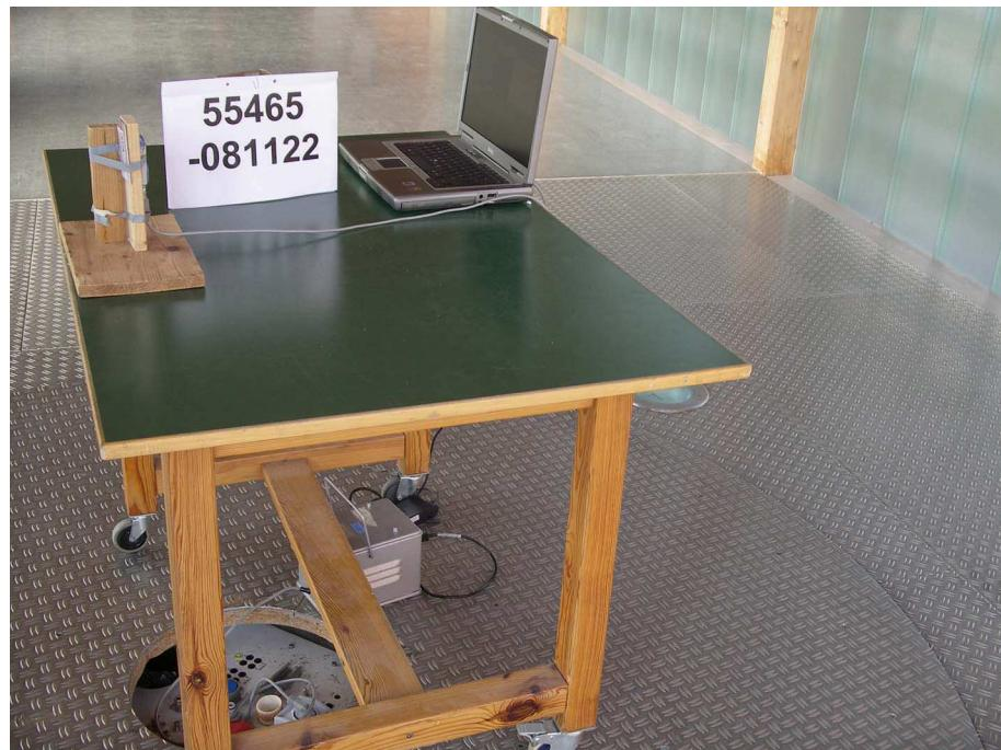
**Test setup for radiated emission measurement
