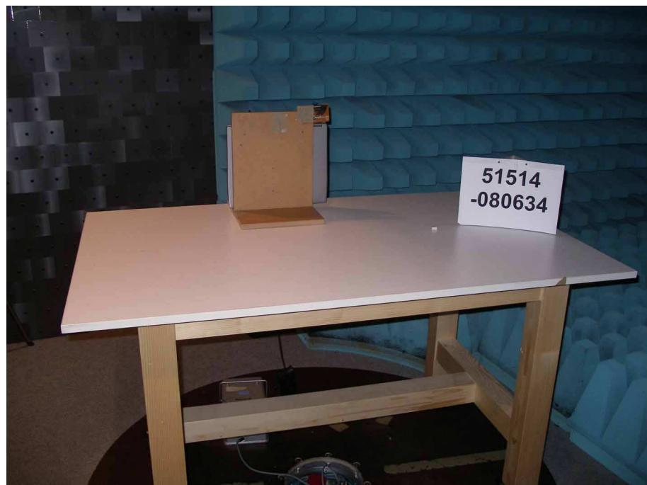
**Test setup for radiated emission measurement
