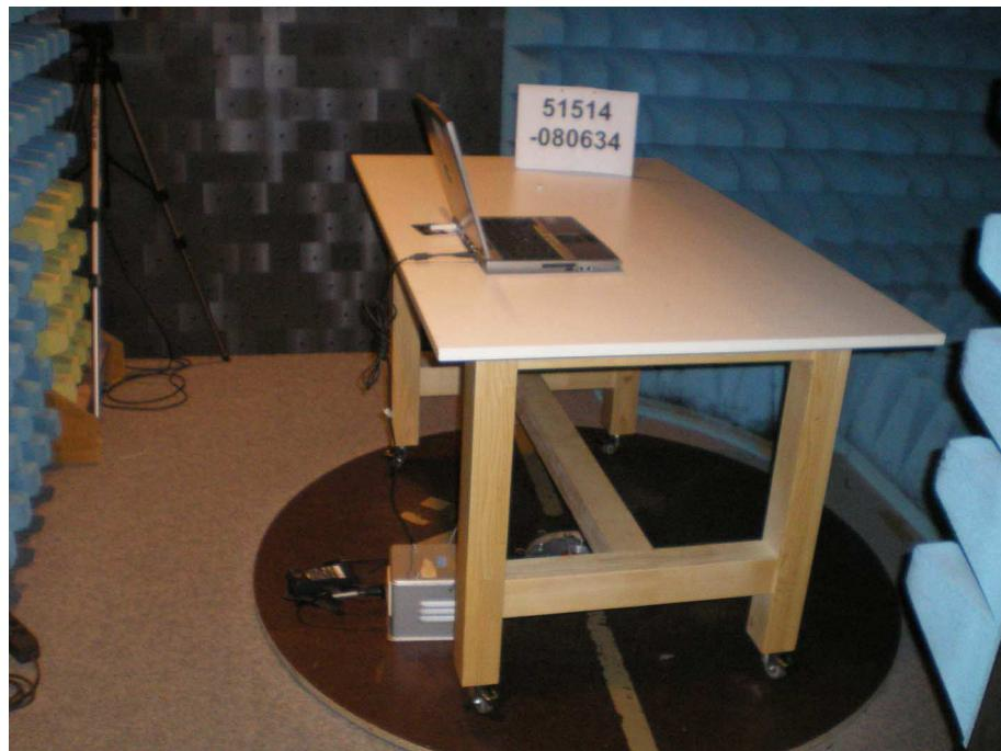
**Test setup for radiated emission measurement
