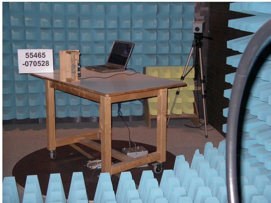
**Test setup for radiated emission measurement
