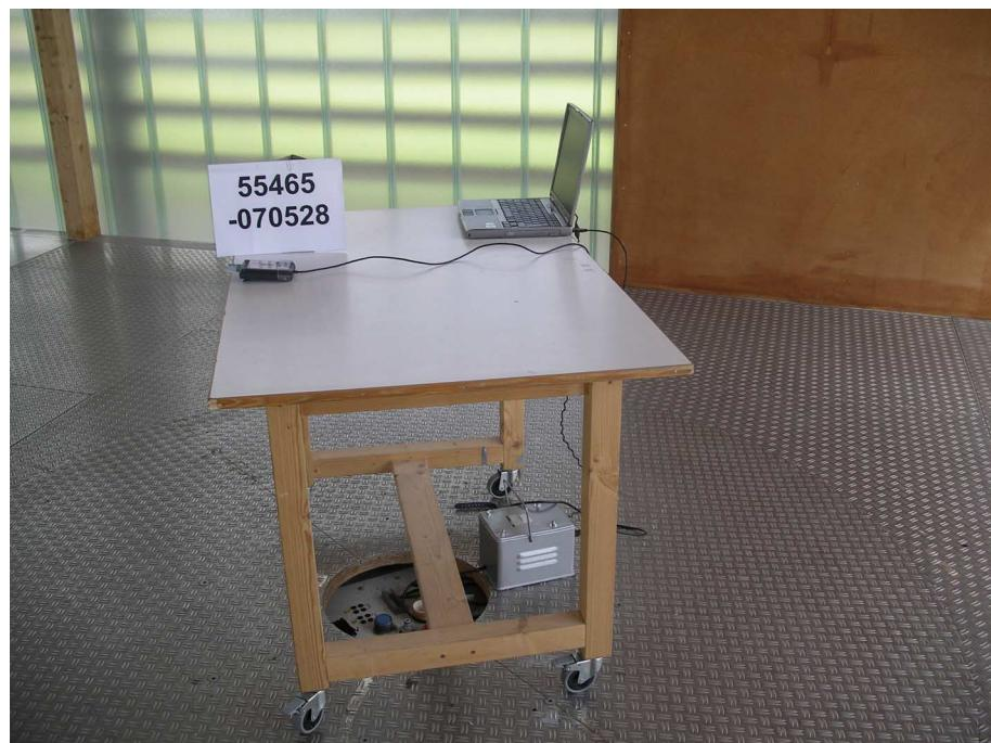
**Test setup for radiated emission measurement
