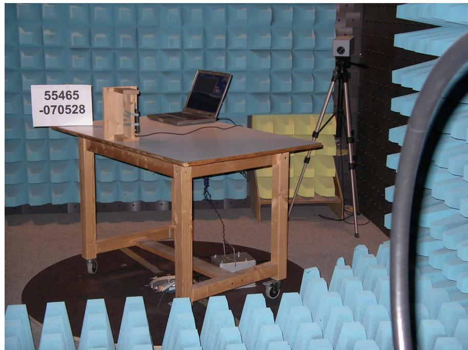
**Test setup for radiated emission measurement
