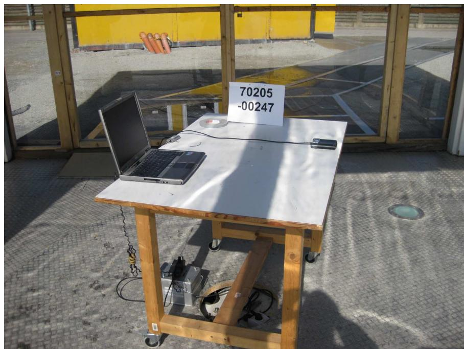
**Test setup for radiated emission measurement
