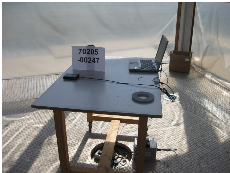
**Test setup for radiated emission measurement
