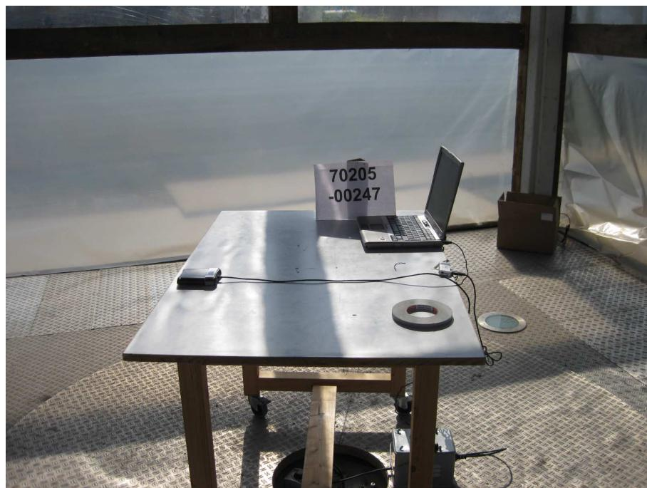
**Test setup for radiated emission measurement
