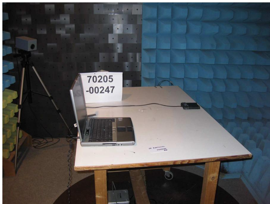
**Test setup for radiated emission measurement
