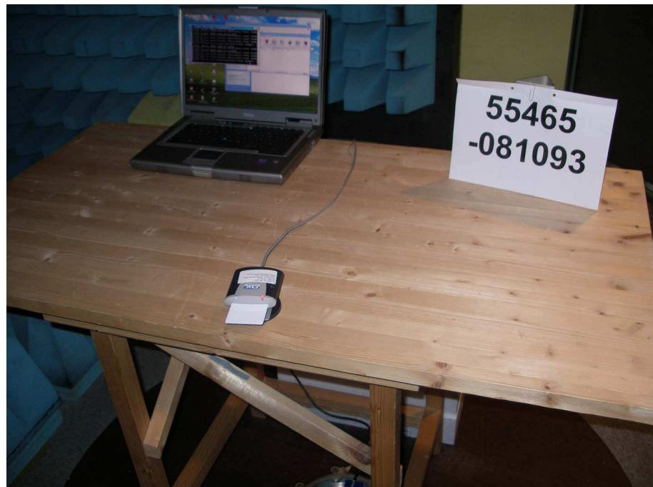
**Test setup for radiated emission measurement
