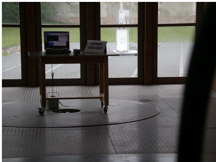
**Test setup for radiated emission measurement
