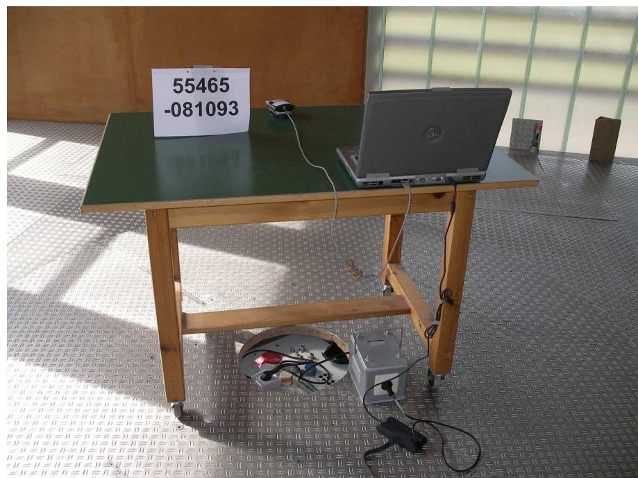
**Test setup for radiated emission measurement
