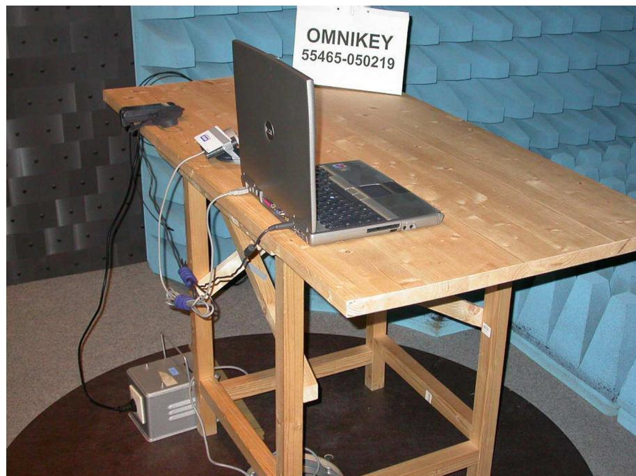
**Test setup for radiated emission measurement
