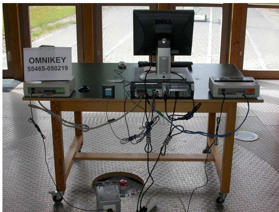
**Test setup for radiated emission measurement
