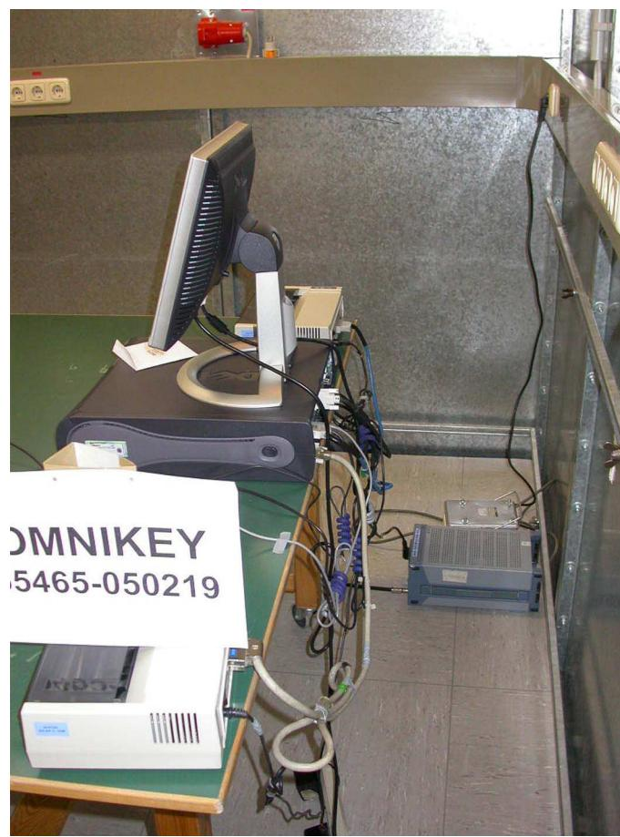
**Test setup for conducted AC powerline emission measurement**
