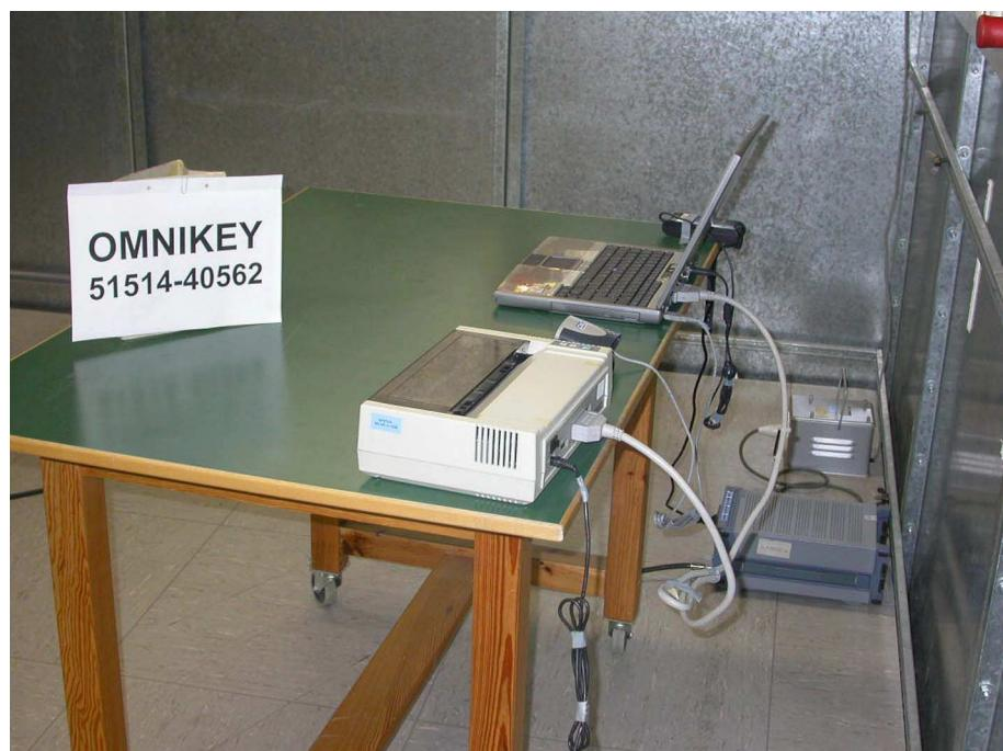
**Test setup for conducted power line emission measurement**
