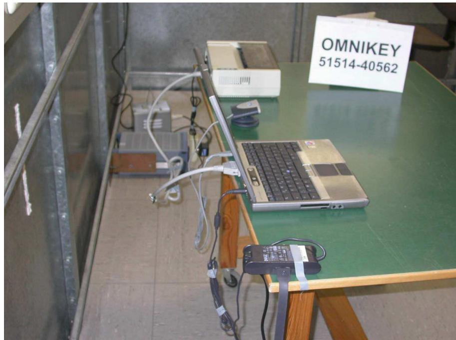
**Test setup for radiated emission measurement
