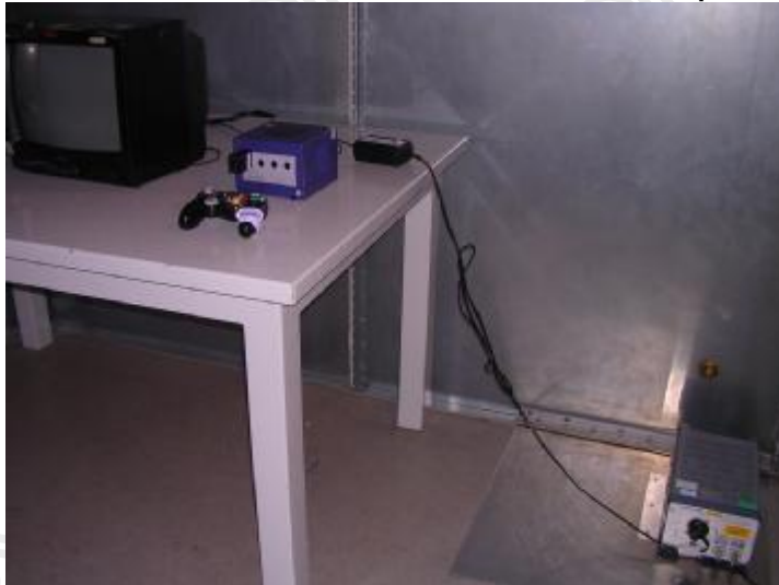
Measurement of Conducted Emission Test Set Up
