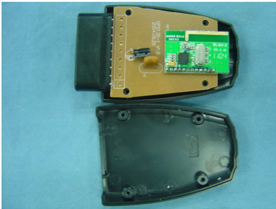
Figure 4 Main Board, Component Side
