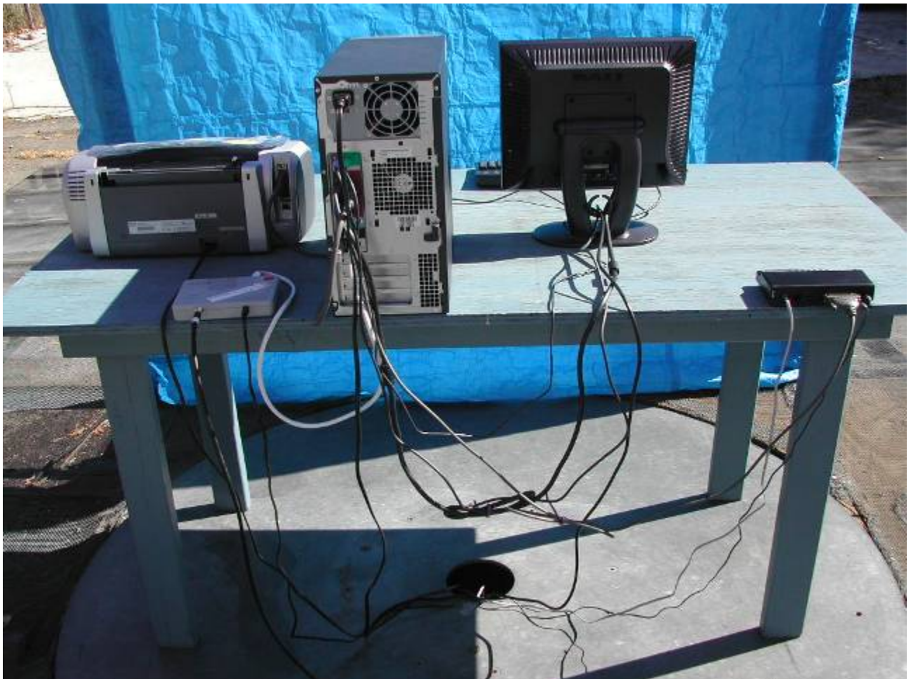
FIGURE 2: PLI Photograph Number 5406C3334SJ-09 illustrates the rear view of the Equipment Under Test with all peripherals attached during the "open field" Radio Frequency Interference / Electromagnetic Interference test program.
