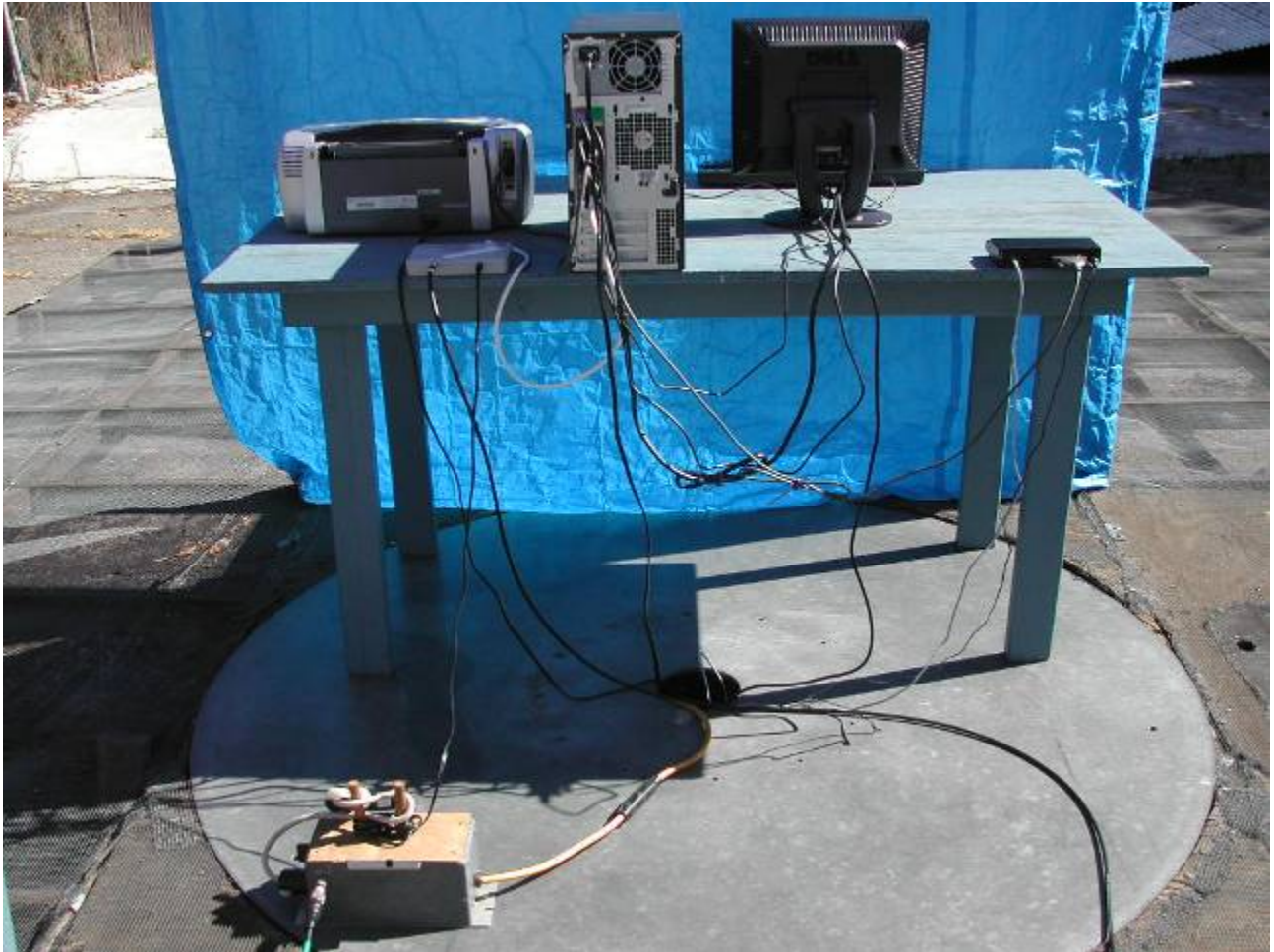
FIGURE 3: PLI Photograph Number 5406C3334SJ-10 illustrates the rear view of the Equipment Under Test with all peripherals attached during the Conducted Electromagnetic Interference test program.
