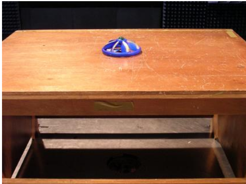
Photo 4: Radiated Emission Test Set-up (Base)
