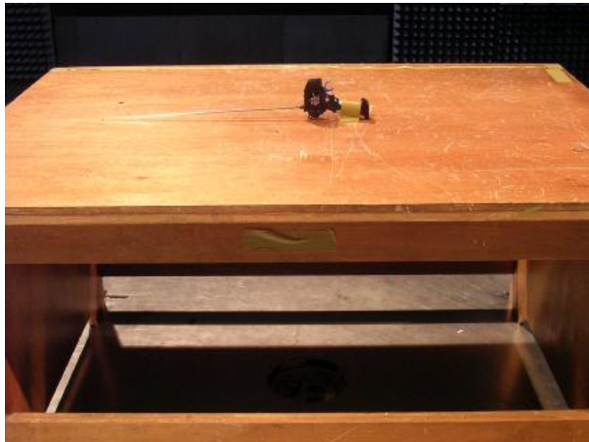
Photo 2: Radiated Emission Test Set-up (Remote control)
