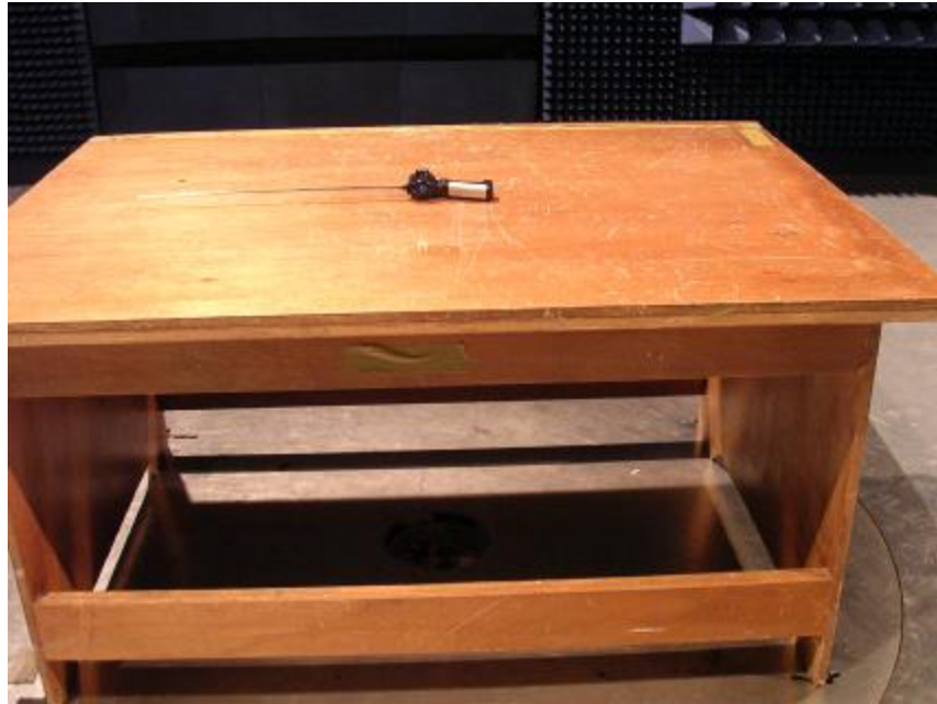
Photo 2: Radiated Emission Test Set-up (Remote control)
