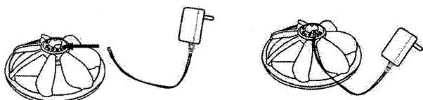
**IMPORTANT:** If the charging nozzle is not completely inserted into the charging cord, the red and green lights won't blink. So should insert again.
