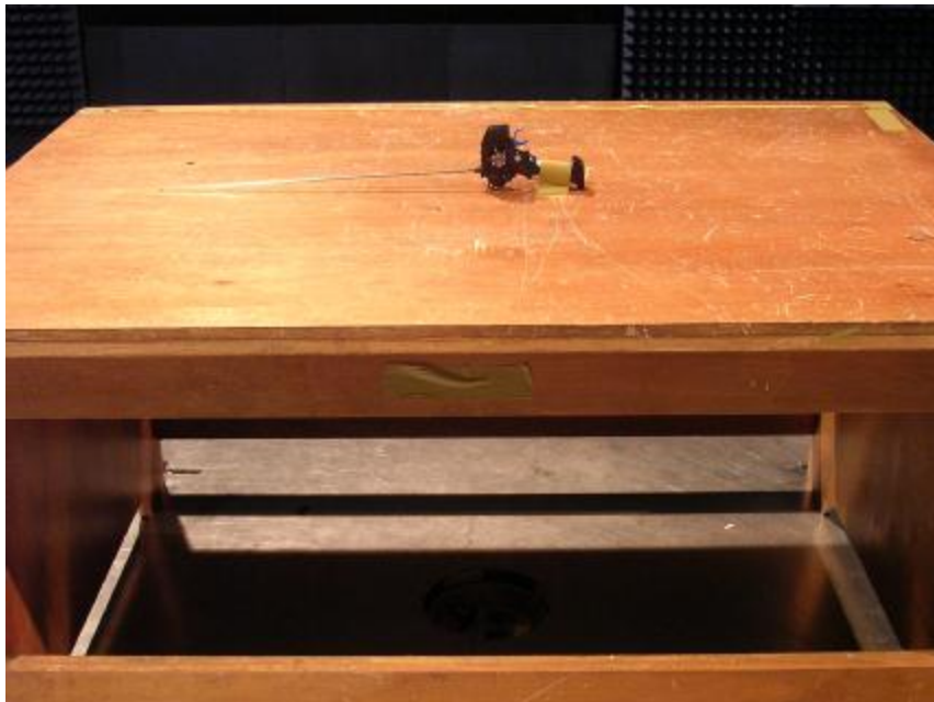
Photo 2: Radiated Emission Test Set-up
