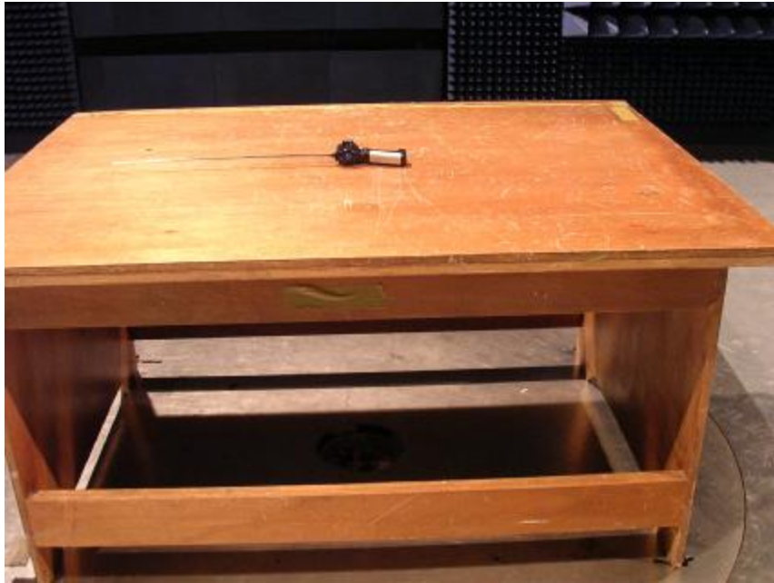
Photo 2: Radiated Emission Test Set-up
