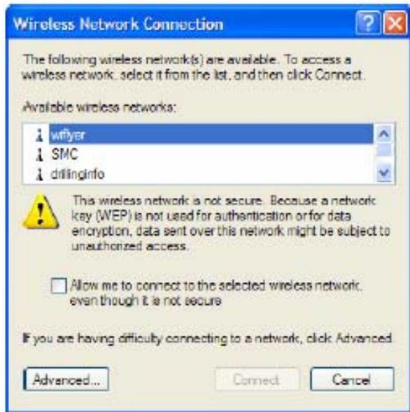
2. Highlight WiFlyer+v, by left clicking it, and check “Allow me to connect to the selected wireless network, even though it is not secure”. To enable security features see Chapter 6.
