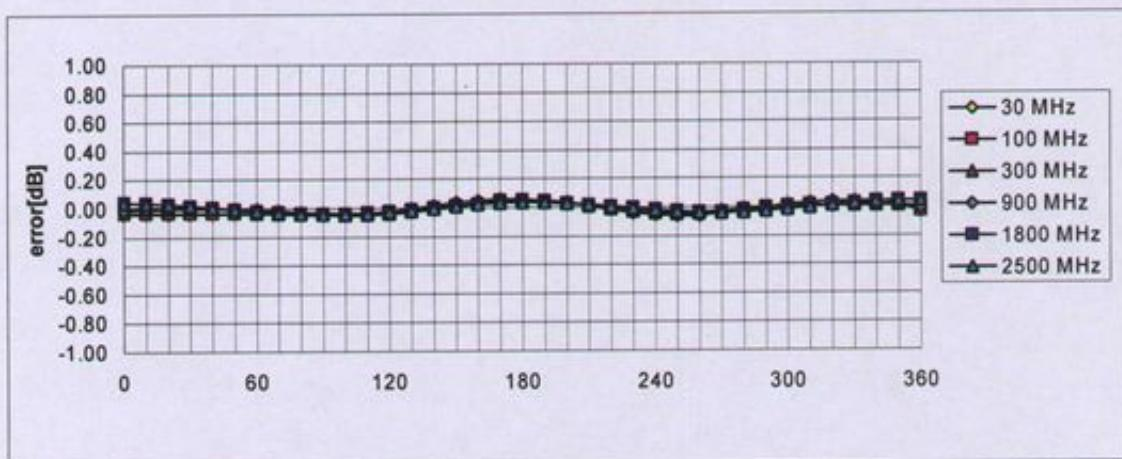
Axial Isotropy Error  $< \pm 0.2$  dB
