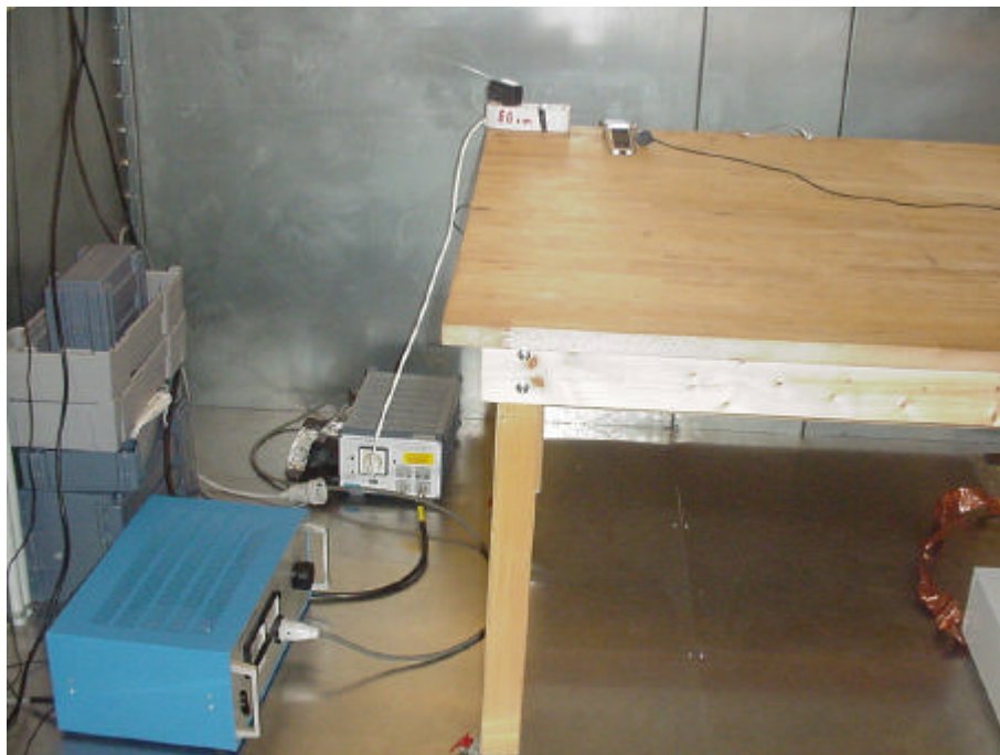
Picture 2 : Setup for conducted emissions tests
