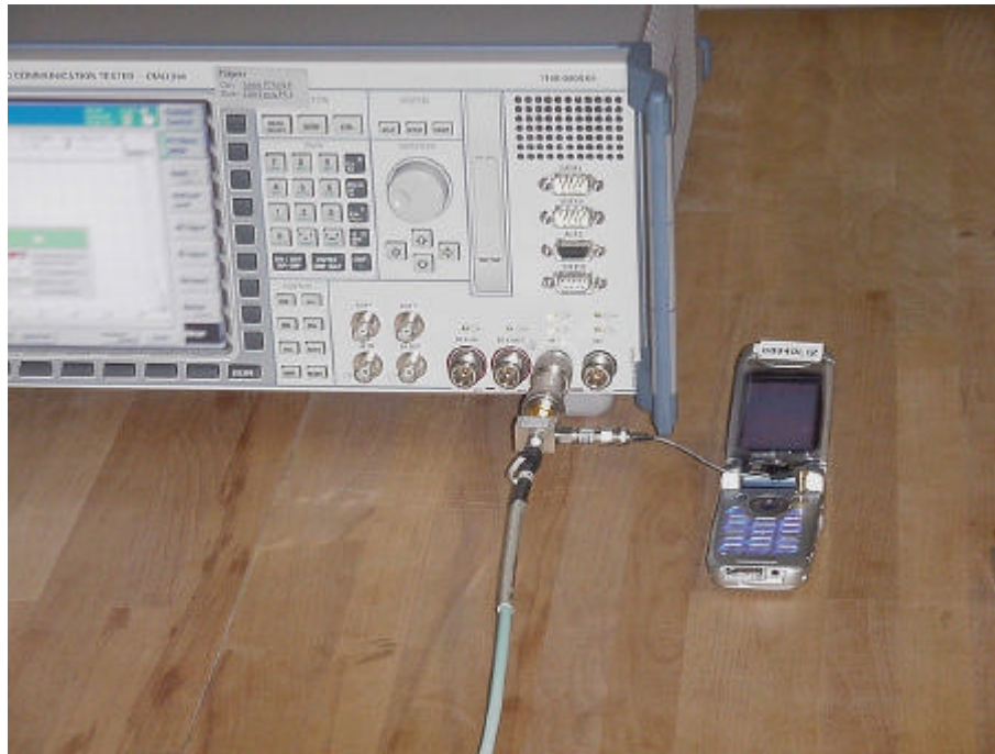
Picture 3 : Setup for conducted tests
