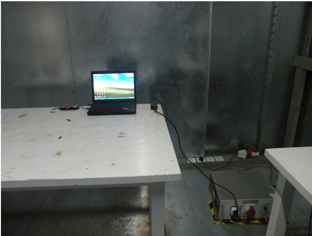
Radiated Emission Test Setup in Chamber
