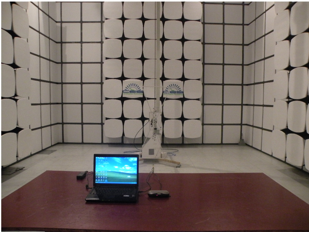
Radiated Emission Test Setup in Chamber
