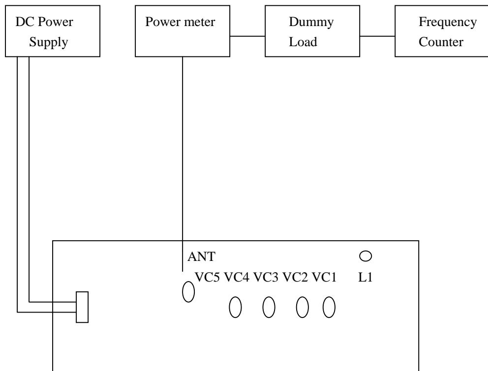
NOTE: The elements illustrated above are solely for explaining the adjustment procedure.
