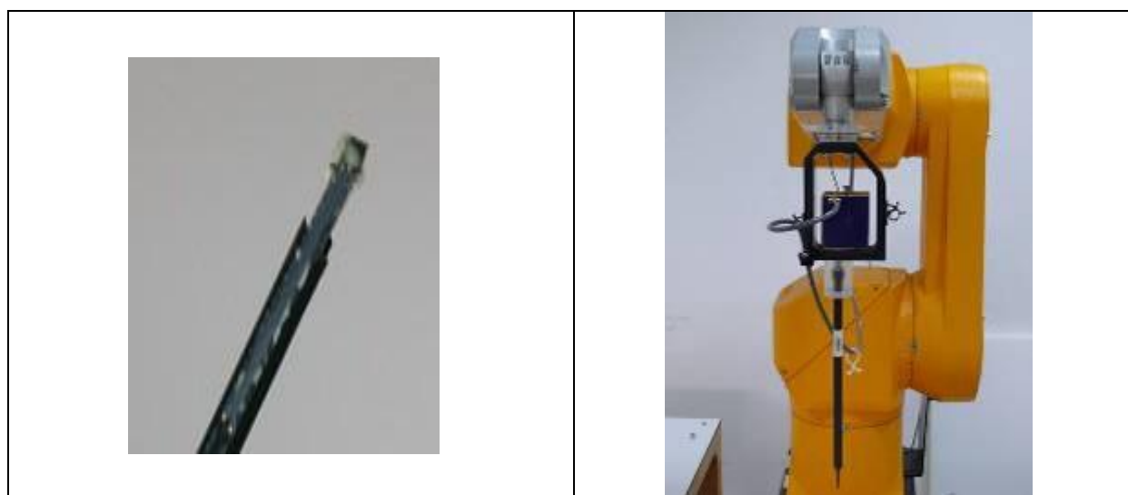
EX3DV4 E-field Probe
