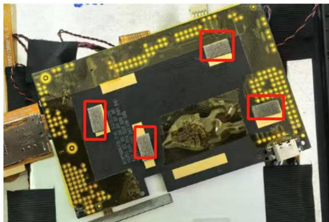
Attach conductive sponge to the marked copper leakage area of the motherboard and ground it to the screen
