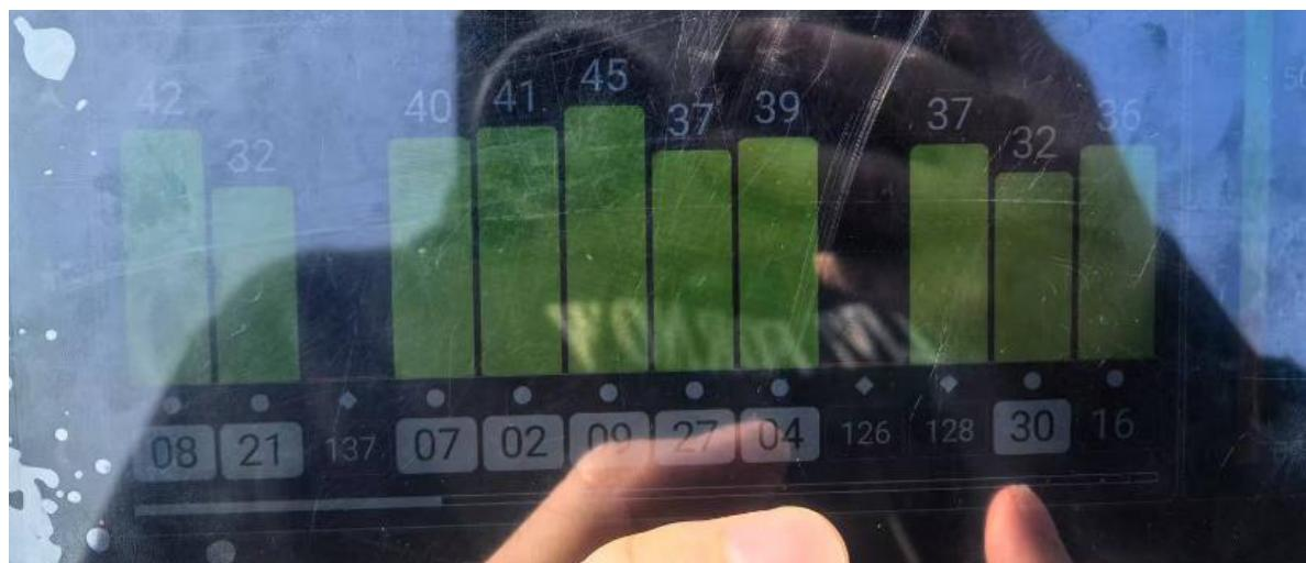
Tested on the rooftop of the fifth floor, the positioning time is about 70 seconds, with a maximum star value of three stars and 40 stars
