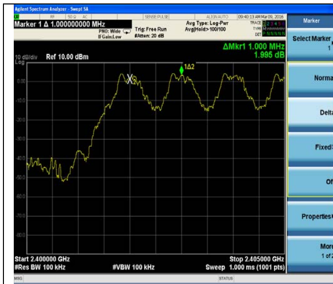
Test Plot Of Frequency Separation (1Mbps)
