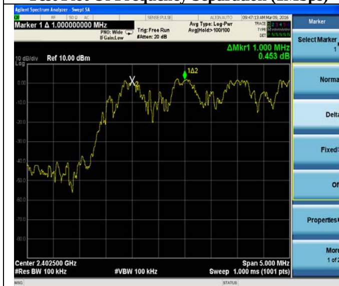
Test Plot Of Frequency Separation (3Mbps)
