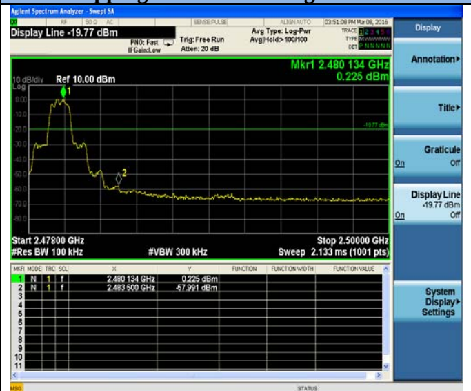
Hopping Off- 8-DPSK-High channel
