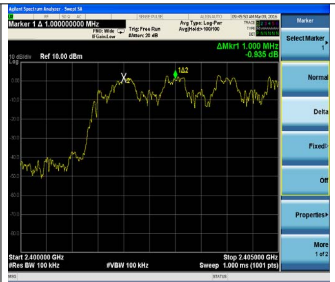
Test Plot Of Frequency Separation (2Mbps)
