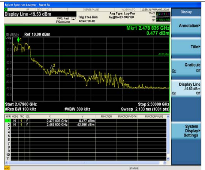
Hopping On- 8-DPSK-High channel
