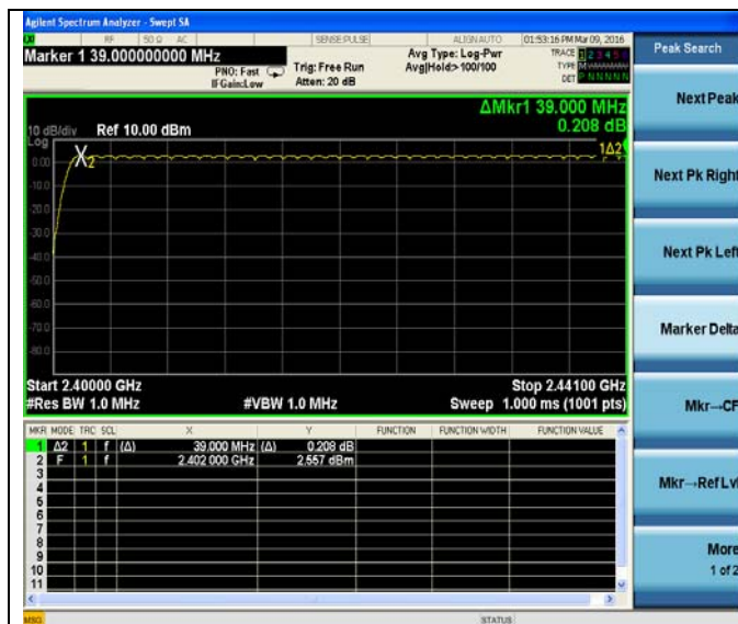
Test Plot 1 For Number of Hopping Channel(GFSK)
