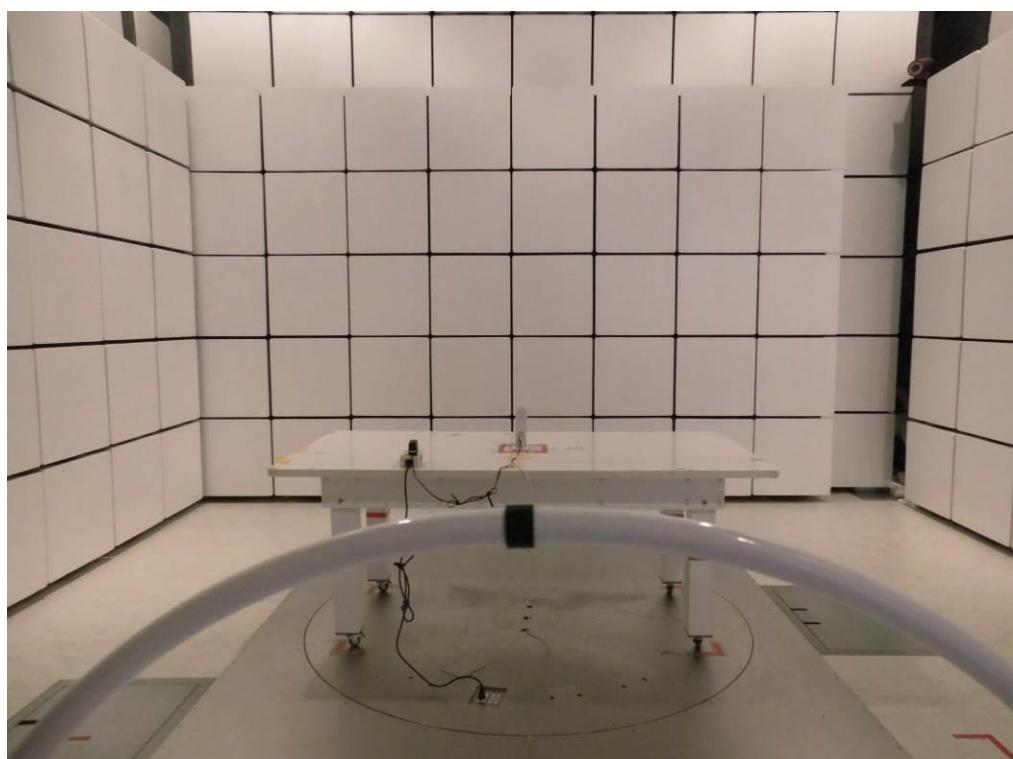
**Radiated Emissions Test Photos****30 MHz to 1 GHz**
