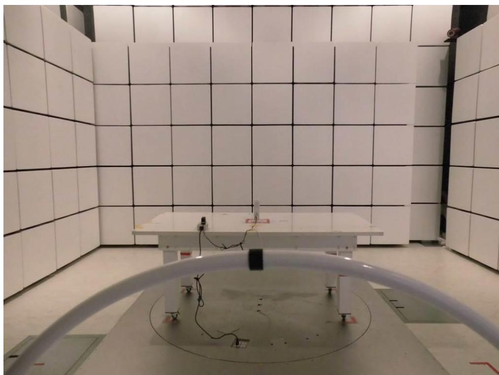
**Radiated Emissions Test Photos****30 MHz to 1 GHz**
