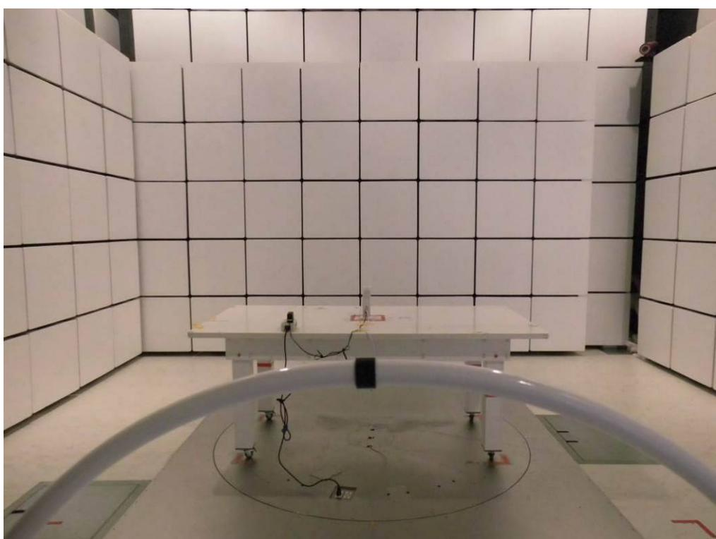
**Radiated Emissions Test Photos****30 MHz to 1000 MHz**
