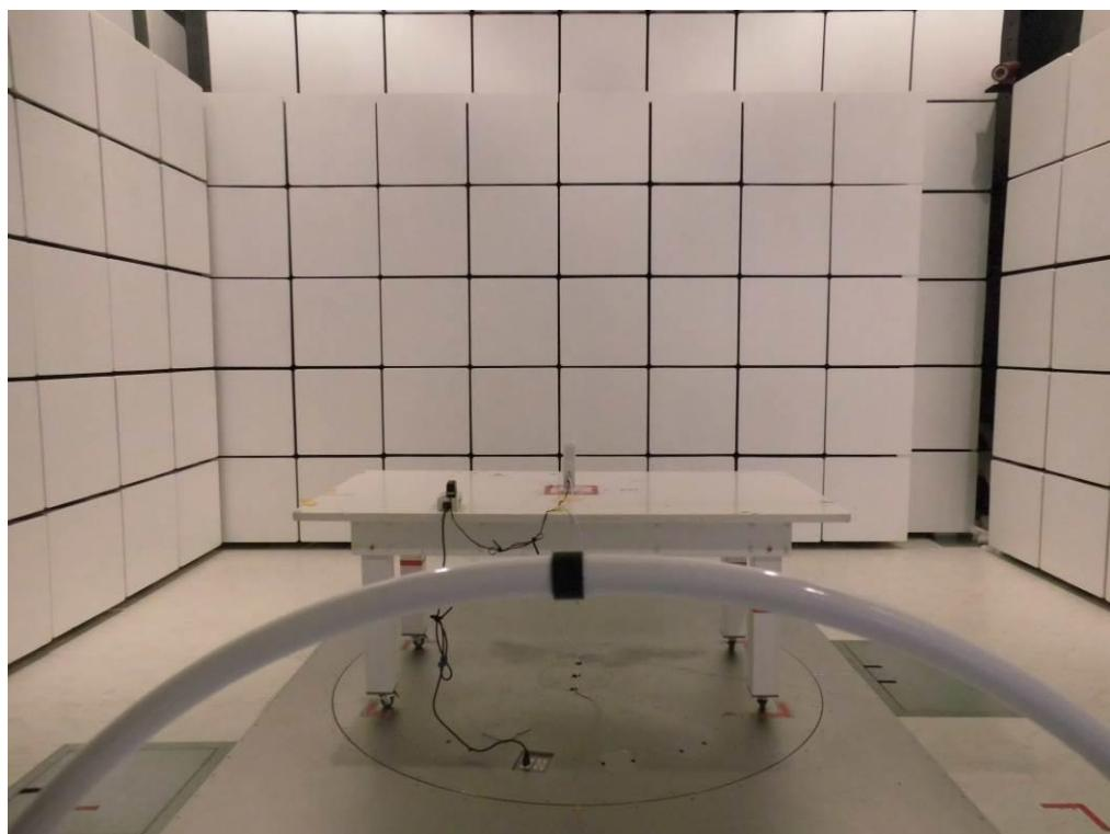
**Radiated Emissions Test Photos****30 MHz to 1000 MHz**
