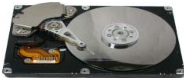
Figure 2. Internal structure of HDD Drive
