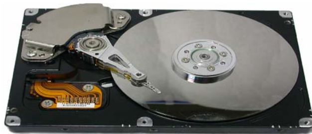
Figure 2. Internal structure of HDD Drive (constructed with flatter disk which stores data and head which read and write the data)
