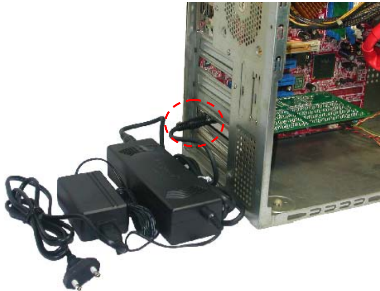
Figure 10. Connecting battery pack to Jet-Speed™
