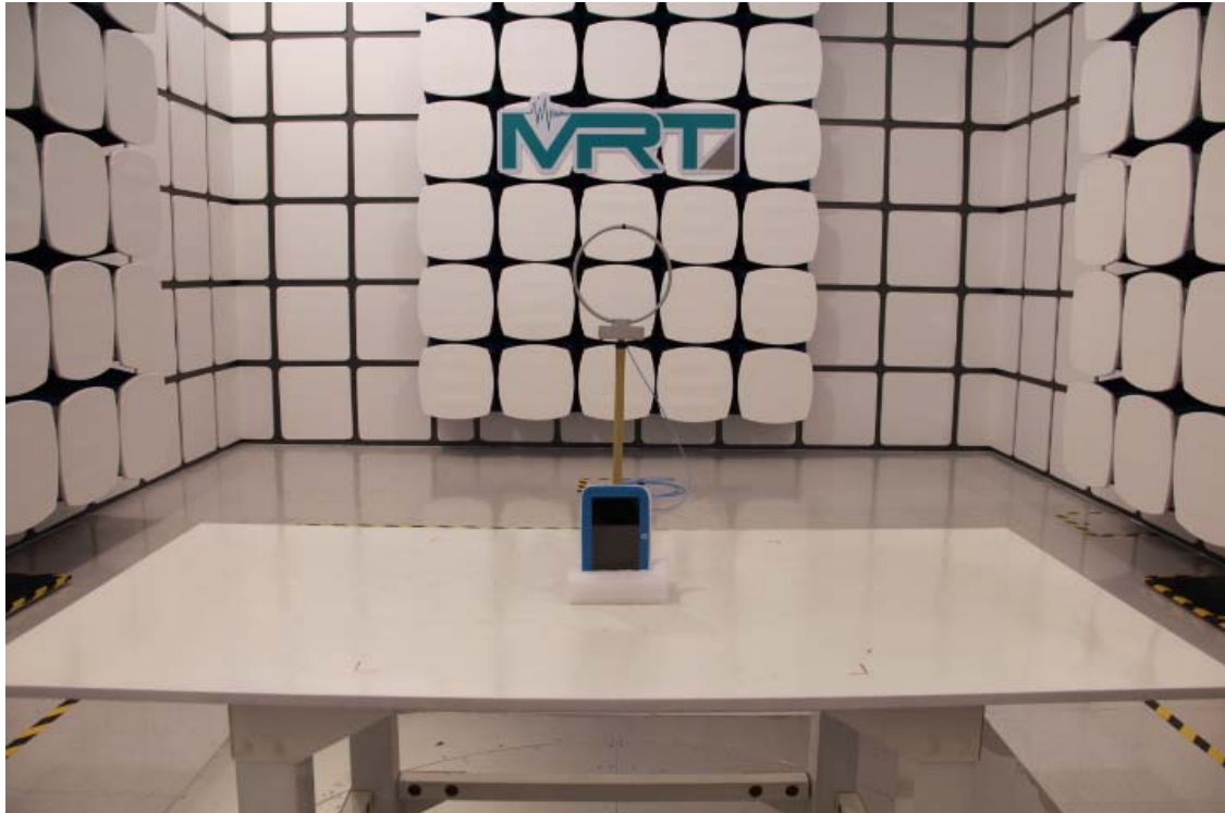
Description: Radiated Emission Test Setup for Below 1GHz
