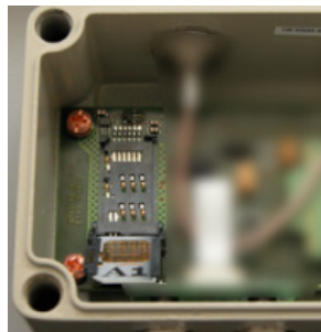
Figure 4. Insert the SIM card into the holder
