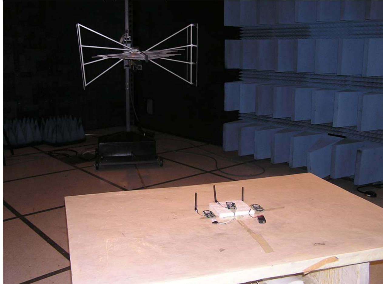
RADIATED EMISSIONS (Dipole Antenna)
