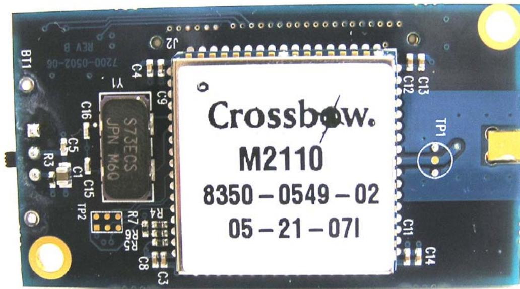
Top Side of Radio Board with RF Shield
