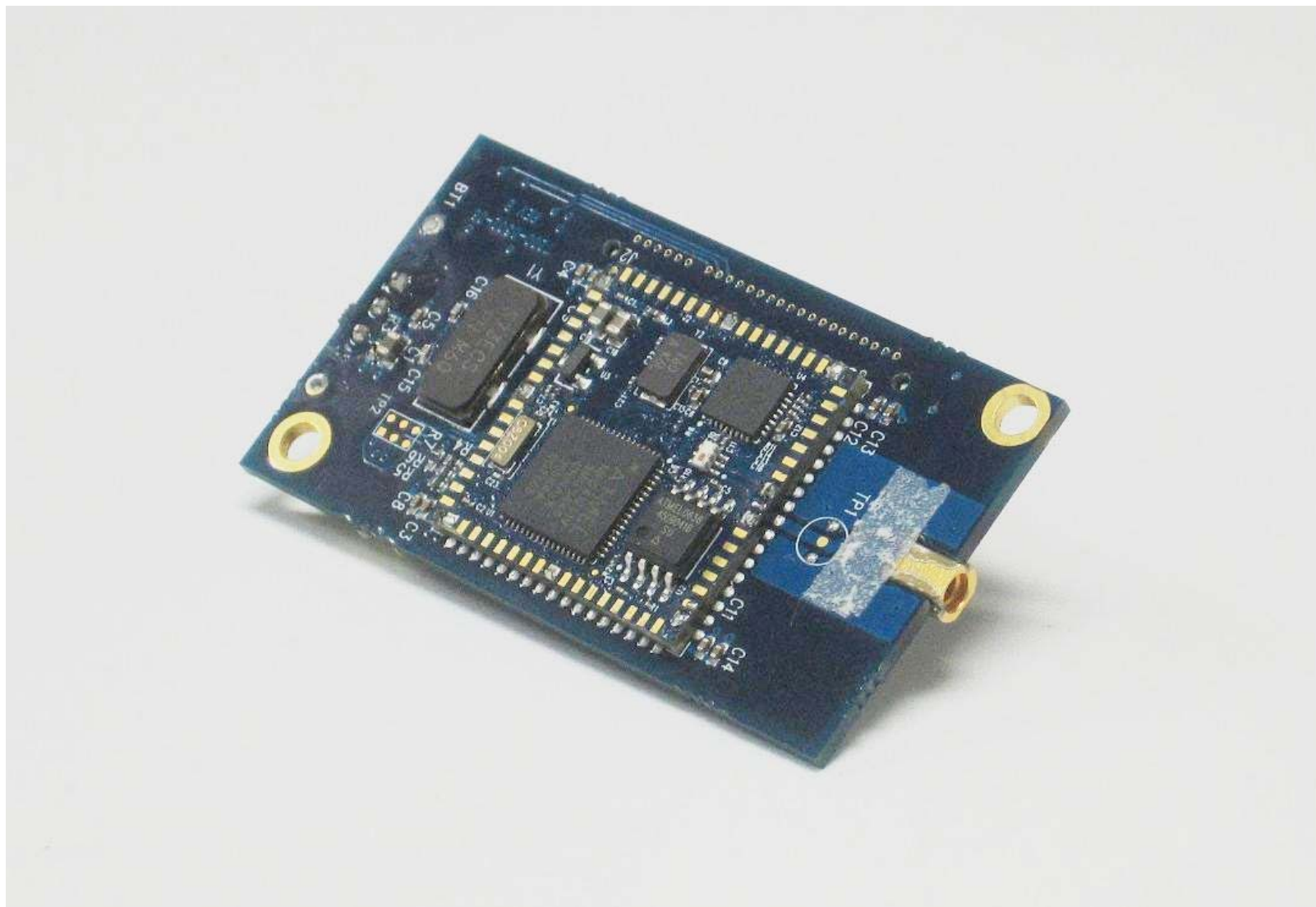
Top side of Radio Board with RF Shield Removed
