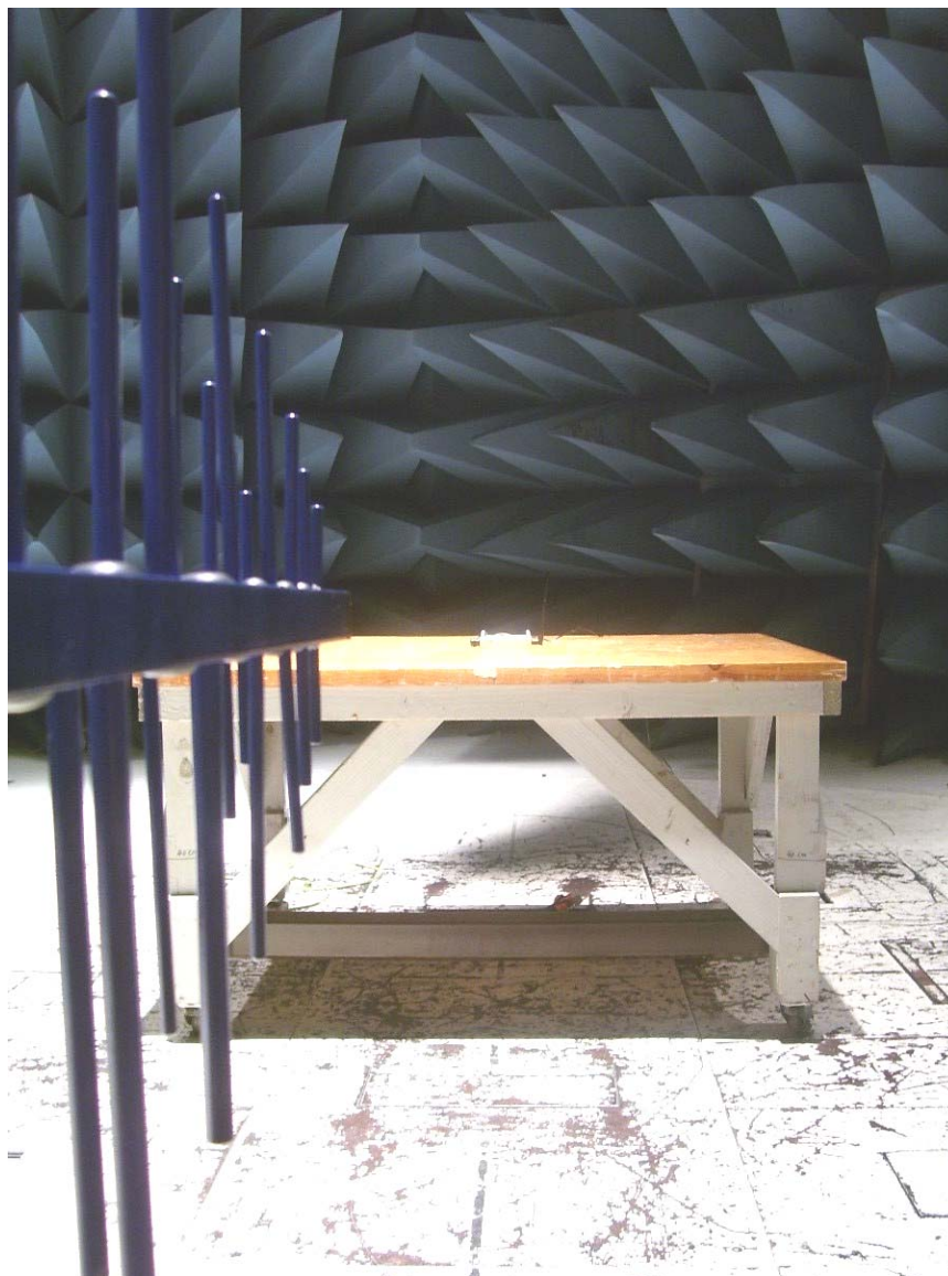
Photograph 5. Radiated Emission Test Setup – Back View
