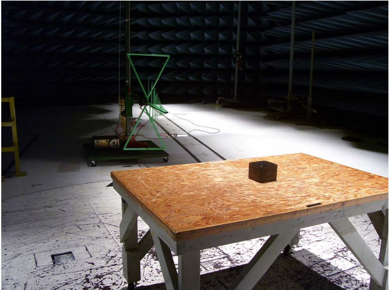
Photograph 2. Radiated Emission Test Setup 30 MHz - 1 GHz
