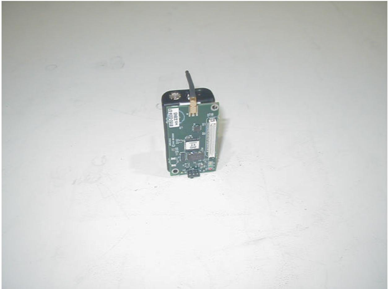
Note – device was tested with batter pack connected but without the outer plastics.
