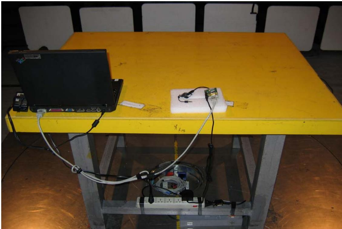
**Radiated Emission Set up Photo (Audio-in Mode)**
