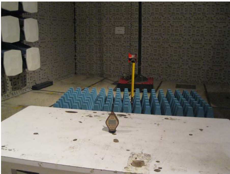
TEST SETUP OF RADIATED EMISSION (1GHz-4GHz)
