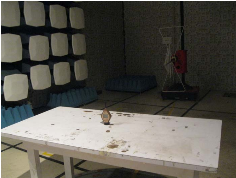
TEST SETUP OF RADIATED EMISSION (30MHz-1GHz)
