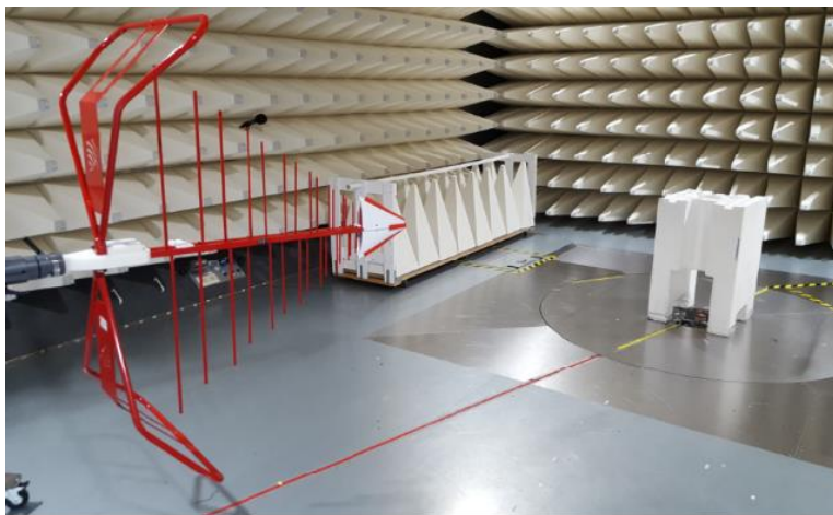
Figure B5. Radiated Test Setup 1
